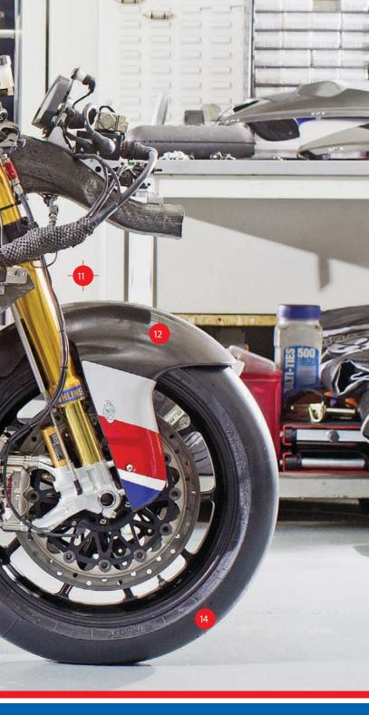
£16,500 initially to have the moulds made. The shape is based around a Moto2 fairing, though increased in size and tested for aerodynamics using computer software by PES Performance. The front mudguard is taken from Paul Bird's MotoGP bike while the hugger is adapted from a WSB ZX-10R unit.
