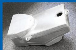
➤ The carbon tank cover is a dummy and literally keeps the lid on a huge airbox
