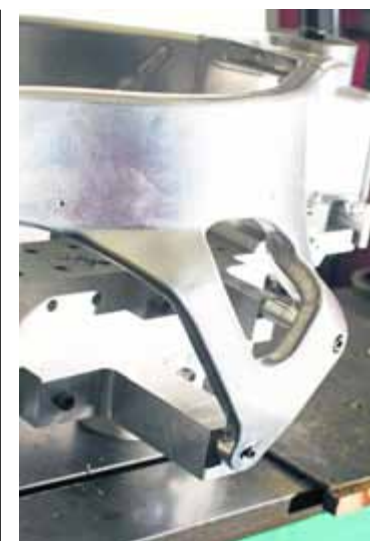
High accuracy means once in the jig there's minimal welding distortion
