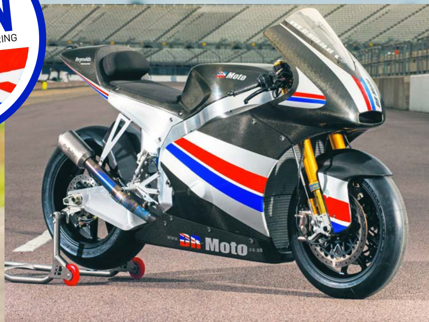
Billet aluminium frame, carbon-fibre bodywork and 198bhp justifies the £90,000 pricetag
